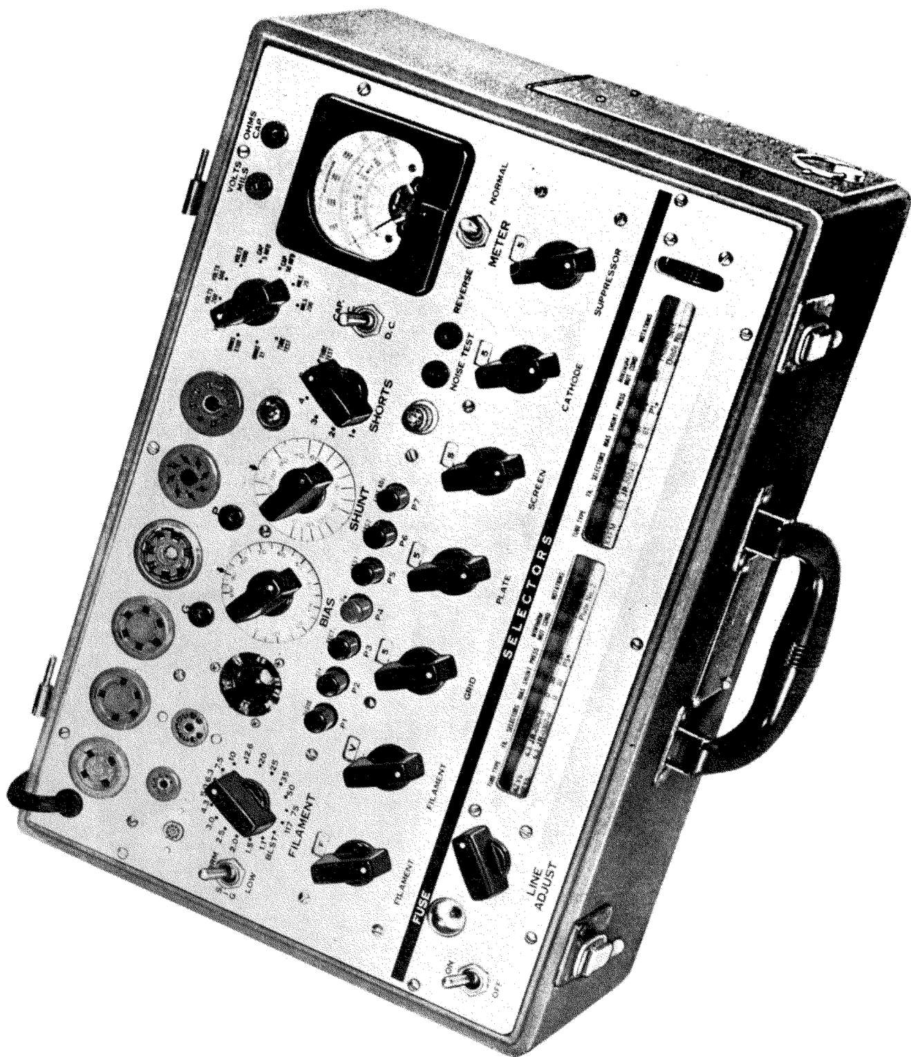
Figure 1-1. Tube Tester TV-3/U with Cover Removed
